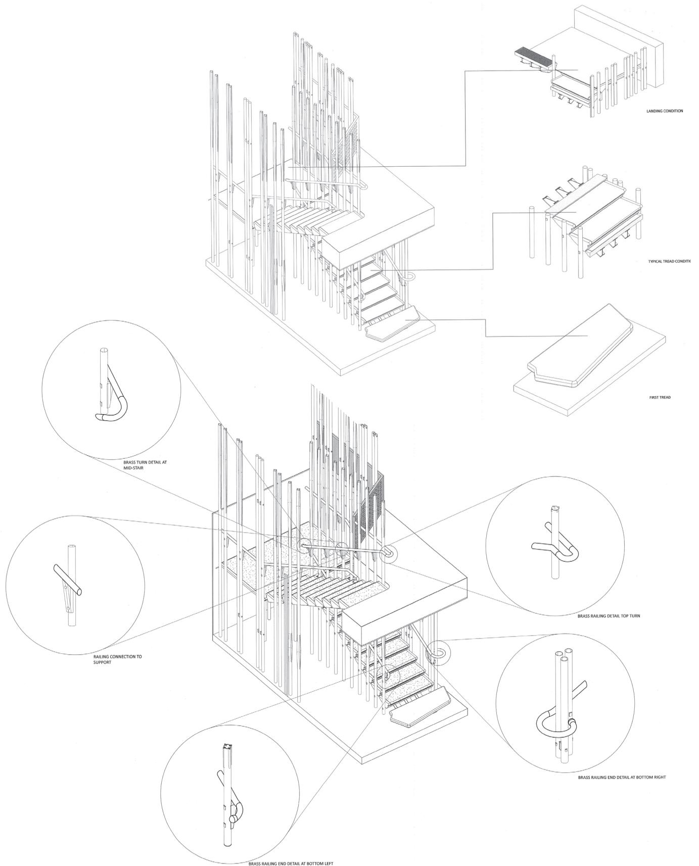
Figure 4: Digital reconstruction of Villa Mairea main stair in Revit
